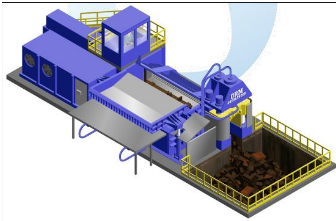
Figure 5: Graphic illustration of baling plant
